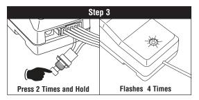
Push the receiver button 2 more times, holding on the last push. The LED will flash 4 times indicating that all remote codes are cleared.
