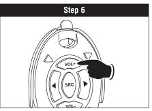
Try each button on the remote to make sure each button has been learned properly. If the remote does not function properly proceed to "Manual Code Learning" section below.
