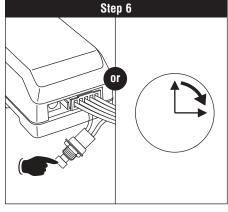
To exit programming push the switch on/off 3 times or wait 15 seconds and the system will automatically exit the "Manual Code Learning" mode.
