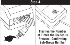
Press the switch on/off the number of times according to the radio manufacturer's **Group** number listed in the Manufacturer's Code Look-Up Table.
