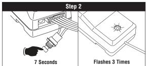
Press and hold the button on the receiver for **7** seconds. The LED on the receiver will flash 3 times and then turn off. Release the switch. You are now in "Manual Code Learning" mode
