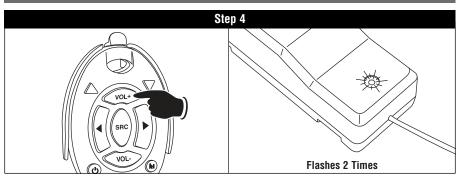
Using the RF Marine Remote press the corresponding "VOLUME UP" button to assign this function.
