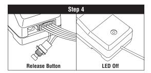
Release the receiver's button and the LED will turn off.
