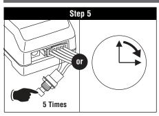
To exit programming push the switch on/off 5 times or wait 15 seconds and the system will automatically exit the "Automatic Code Learning" mode.
