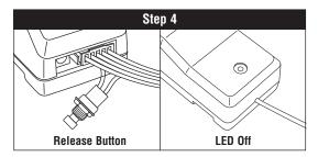
Release the receiver's button and the LED will turn off. Repeat Steps 2-4 to program additional remotes.
