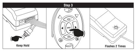
While still pressing the button on the receiver, press and release the SRC button on the remote until the LED on the receiver flashes 2 times, indicating the code is learned.
