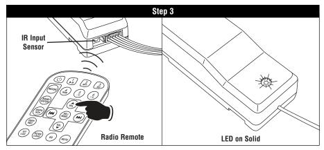
Within 15 seconds, aim the radio remote at the IR input sensor and push the "VOLUME UP" button on the radio remote.
